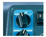
Auto High: High mode provides maximum rim pull and fast cycle times by shifting the transmission at high engine speeds. This mode is suitable for hill-climb and load and carry operations.
